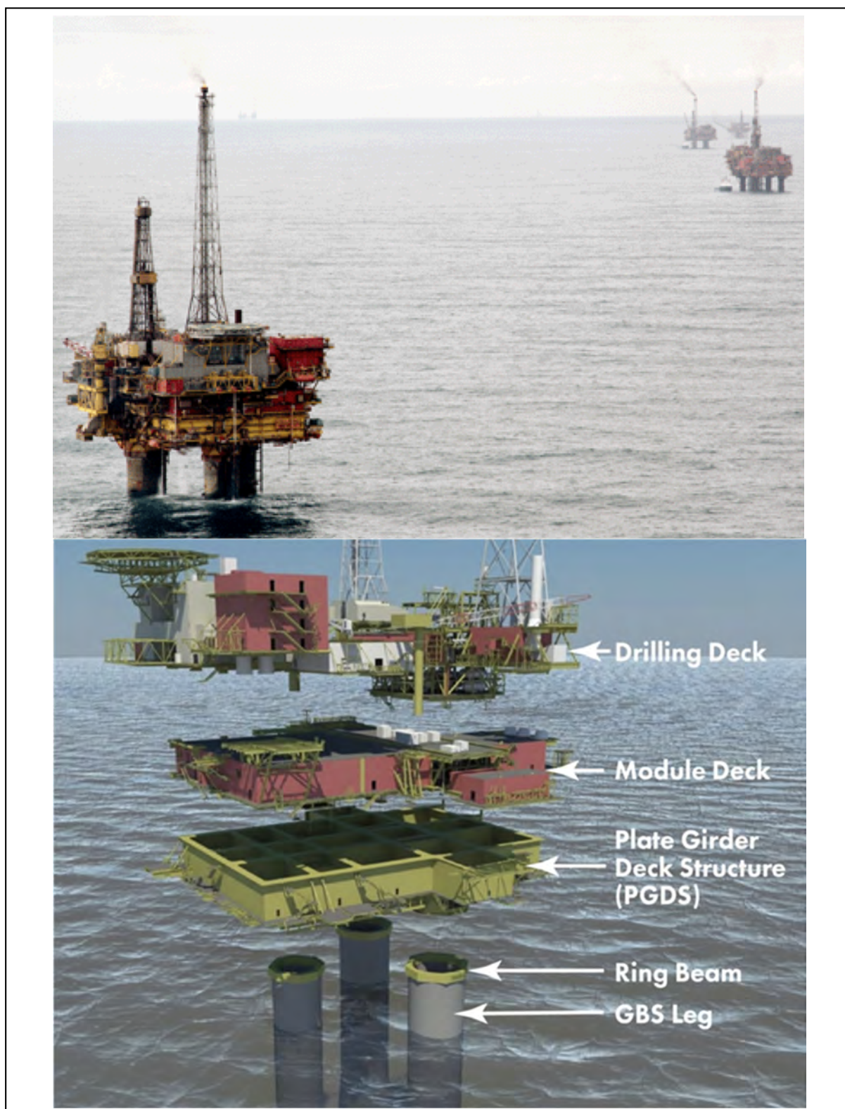
Figure 8-4: Brent D Topsides General Configuration
