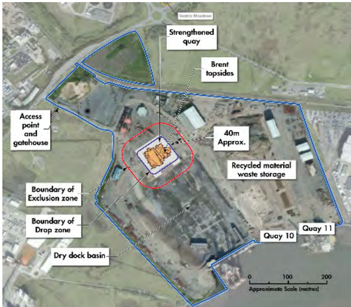
Figure 8-16: Plan of Exclusion Zone around Topsides
