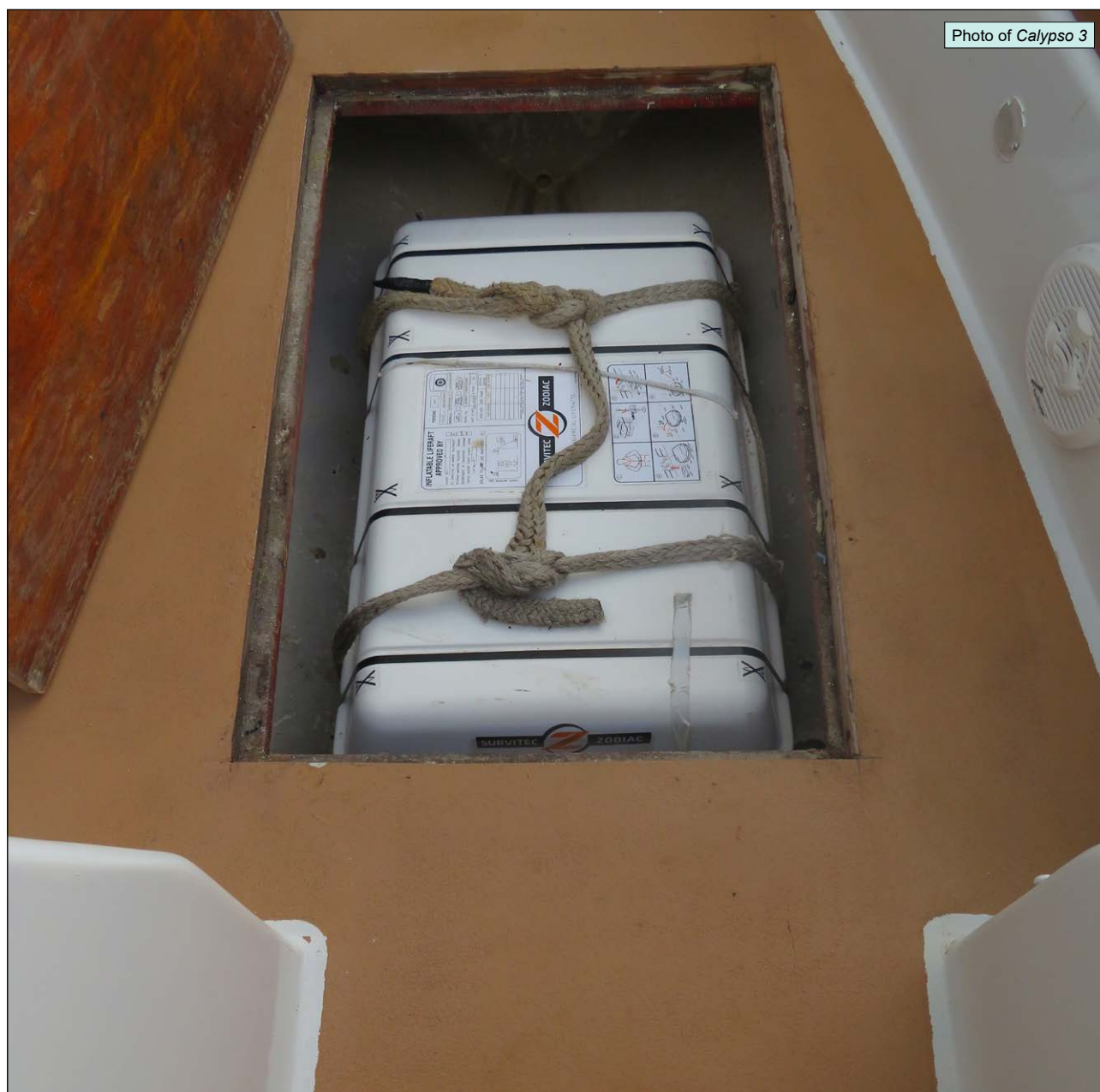
Figure 8: Liferaft stowage in the foredeck seating area
